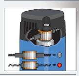
The machines of the Profi-PLUS class are provided with provided with an indicator to visualise & control the wear of the carbon brushes. By replacing the worn carbon brushes in time, you will protect the motor of your machine from damage.
