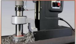
Magnetic core drilling with large calibres. Up to 130 mm in diameter and up to 110 mm cutting depth - a comparison of all BDS machines can be found on pages 10-11 and 46-49, along with the complete BDS core drilling range.
