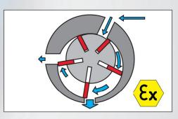
AirMAB 5000 – magnetic core drilling with pneumatic drive. The high performance vane motor performs at 830 Watt and is approved according to Ex class - Ex II 2G T4 IIC D110° C.
