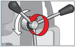
MAB 1300 – drilling with servo-assistance. PowerASSIST is a power-assisted feed when drilling - a particularly welcome aid for core drilling with large diameters.
