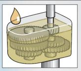
One of the most important and differentiating feature of a BDS magnetic core drilling machine is its gearbox. The BDS machines have multi-stage oil gearbox. An oil gearbox helps in provding lubrication to all the gears uniformly, therefore making the BDS machines more robust and reliable for longer service time.
